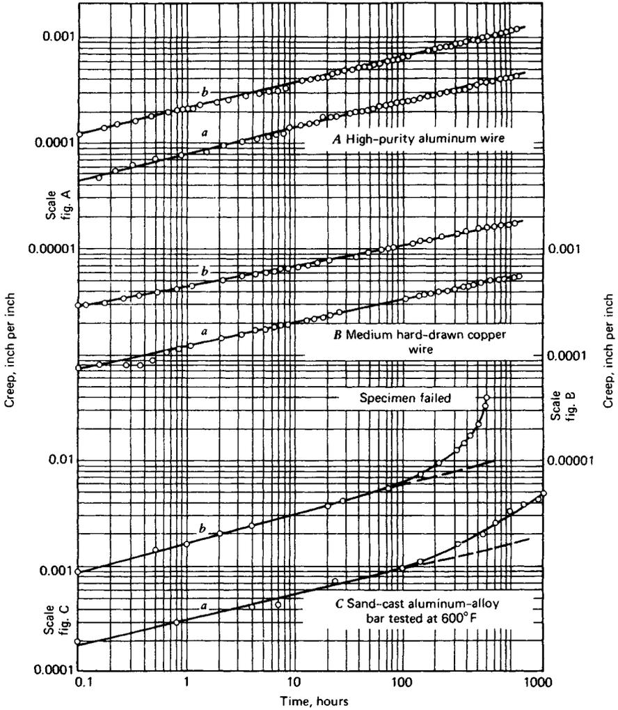
Fig. 18.63 Creep curves for three materials plotted on log-log coordinates. (From Ref. 77.)
