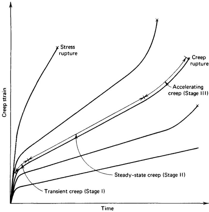
Fig. 18.62 Illustration of creep and stress rupture.
